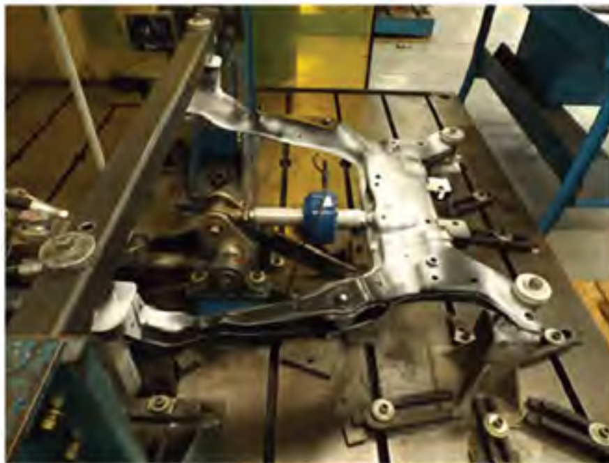
Figure 8: roll restrictor test setup
