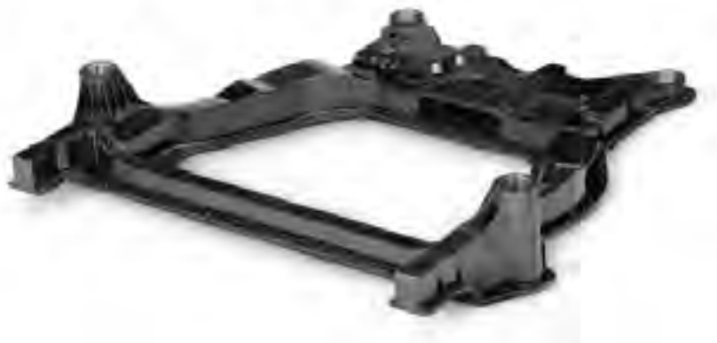
Figure 7: CF composite subframe prototype part
