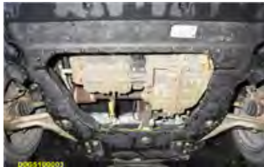
Figure 18: CF subframe – post vehicle durability test
