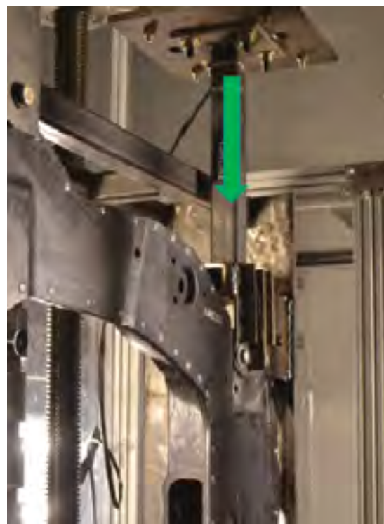
Figure 28: Strength test – control arm rear joint loading
