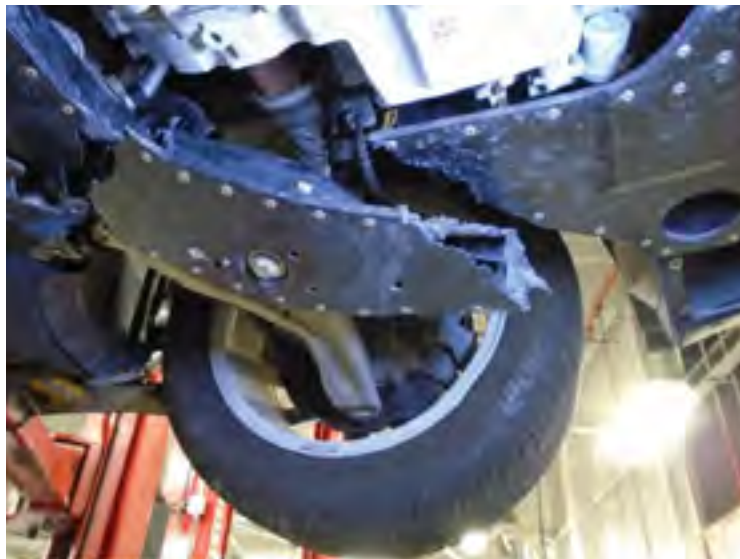
Figure 32: CF subframe – post vehicle special event test
