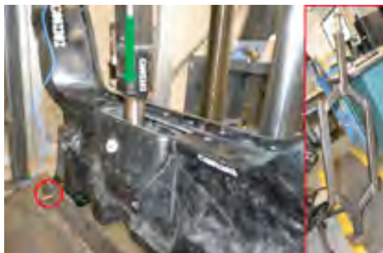
Figure 20: Strength test – roll restrictor loading
