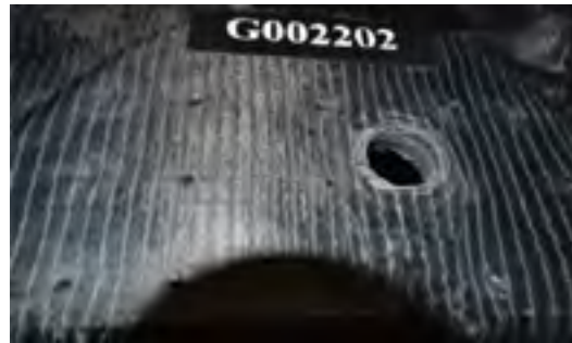
Figure 21: strength test – roll restrictor loading damage
