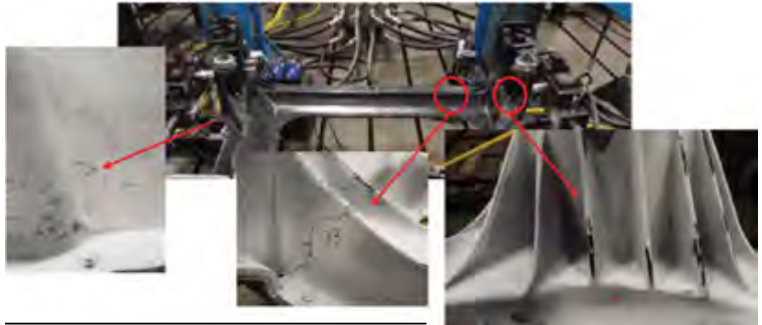
Figure 12: control arm test cracks –CF subframe
