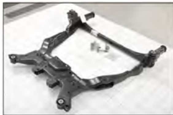
Figure 1: Ford Fusion steel front subframe
