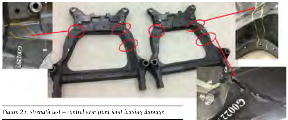
Figure 24: Strength test – control arm front joint loading
