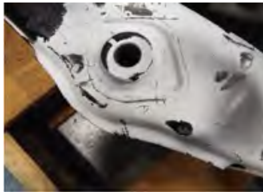
Figure 11: control arm test cracks – steel subframe
