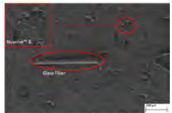
Figure 20: SEM micrograph of 10/10 formulation at 500x magnification
