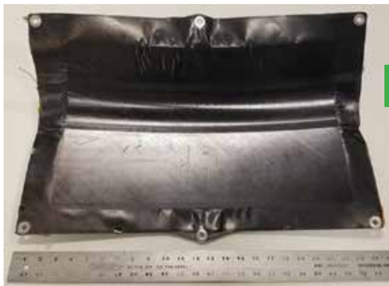
Figure 7 (a) Simulated Aniform displacement results due to the forming process, (b) Simulated Abaqus warpage results adding the effects of heat-transfer, and (c) An as-manufactured part produced at the Purdue CMSC, created using the thermoplastic composites forming process.
