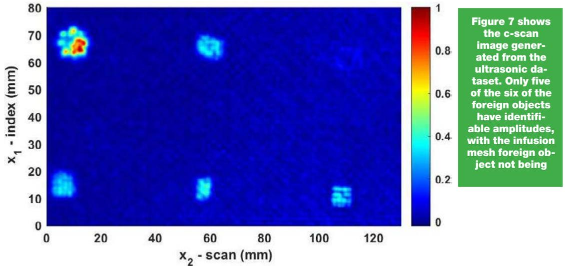
**Figure 7: C Scan plotting the maximum normalized amplitude between the sixth and seventh plies.**
