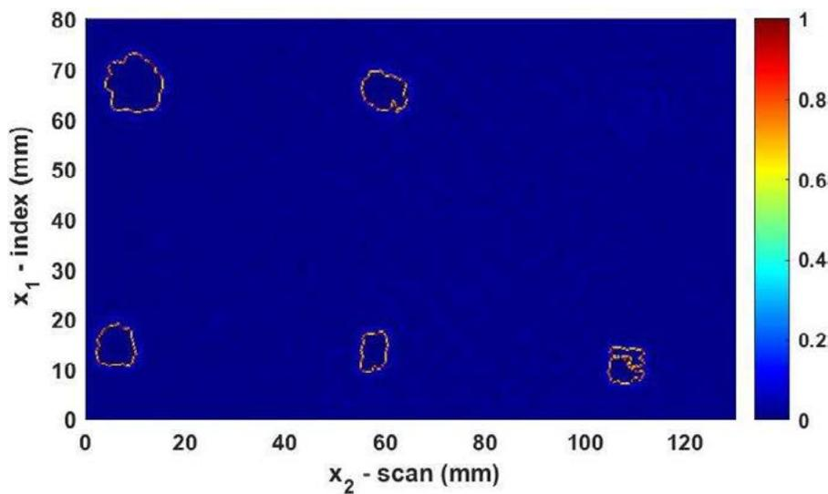
Figure 11: Magnitude of the modified c-scan highlighting the boundaries of the foreign objects.
