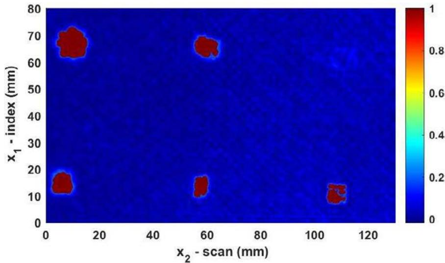
Figure 10: Modified c scan of the amplitudes between the sixth and seventh plies where signals above a threshold are forced to one.
