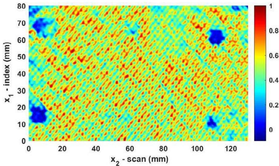
**Figure 8: C** Scan plotting the normalized maximum amplitude across the back wall of the composite.
