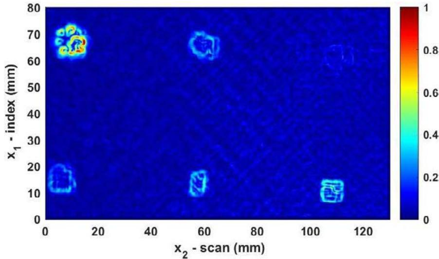
**Figure 9:** Normalized magnitude of the gradient applied to the c-scan between the sixth and seventh plies to determine the edges of the foreign objects.
