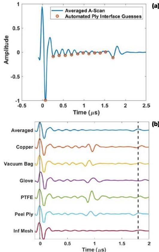
In order to determine the ply interface estimates, shown as the red circles in Figure 4(a), the back wall of the part is first identified, which occurs at approximately 1.8 μs. The number of plies is then determined by the distance in time between the front wall and the back divided by the nominal thickness of an individual ply. The total thickness of the part is identified using the equation:
