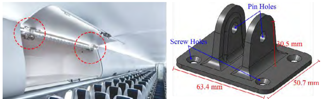
Figure 2: Aircraft overhead bin door pin bracket design.
