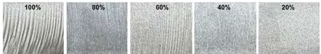
Figure 2. 100% - 20% cutting speeds and the resulting edge surface finish.
